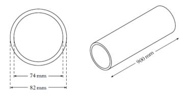
The inner diameter is 74 millimetres. The outer diameter is 82 millimetres. The tube is 900 millimetres long.
